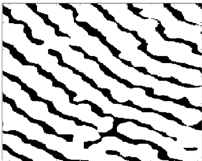
FIG. 6. Representative binary image obtained by processing a TEM image like Fig. 1. The lighter regions have pixel value 1 and represent regions where silver is present (the “wires”). The darker regions have pixel value 0 and represent the exposed PMMA “river” regions. The image represents a field of view about 400\text{ nm} \times 400\text{ nm} .
